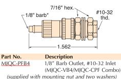
Minimatic J-Series quick connect fittings are very compact yet provide a very high flow. The electroless nickel plated brass body is available with #10-32 threads (M or F), 1/8" NPT threads (M or F), 1/4" NPT threads (M) or a 1/8" hose single barb configuration.
